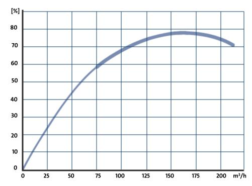
Operation outside bold line limits (75 m³/h and 215 m³/h) is not recommended.
